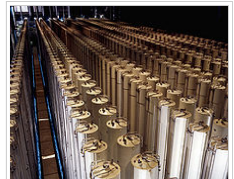
Cascades of gas centrifuges are used to enrich uranium ore to concentrate its fissionable isotopes
