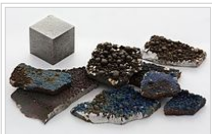
Electrolytically refined manganese chips and 1 cm 3 cube
