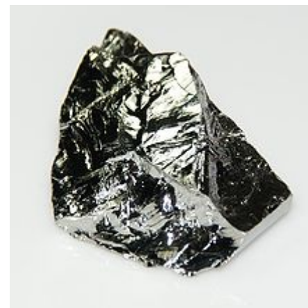
A 12 gram (2×3 cm) polycrystalline block of germanium with uneven cleaved surfaces
